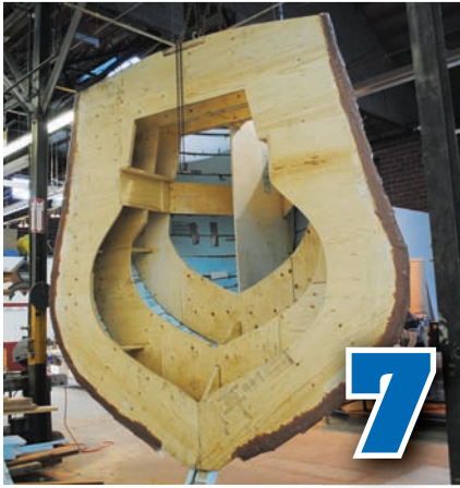
Plywood bulkheads were assembled to create the skeletal shape of the pirate ship.
